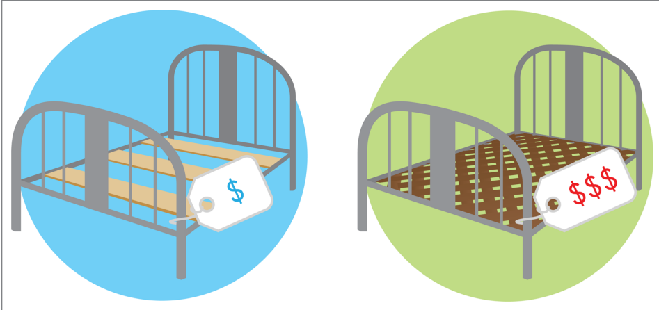
FIGURE 10-4 Balancing robustness and cost. A bed with just horizontal slats (left) is not as strong as a bed with a diagonal grid of slats (right), but the former is less expensive than the latter. Over the years, engineers have repeatedly opted for the less expensive design in this case.
